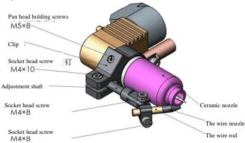
Loosen two M4  $\times$  16 screws, we can make welding torch head's axis and the axis of welded tube of 1~30 degrees angle. In principle, it can achieve making welding torch head's axis and the axis of welded tube parallel and achieve vertical welding of weld plate. The angle of 1~30 degrees is defined as angle adjustment range here. Refer to the table of processing technical for the angle value of specific welding process values.
