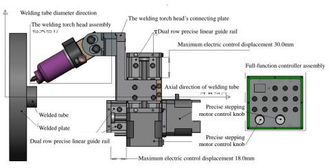
dual guideway with the stainless steel guard can greatly improve the service life of the assembly.
