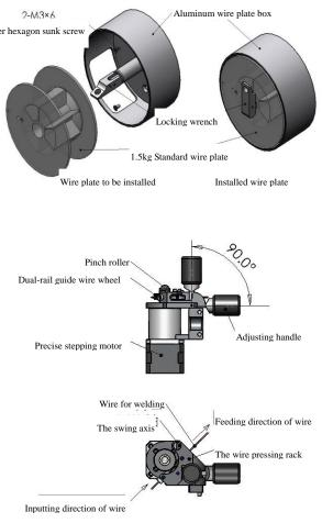
position, appropriately adjust the pressure. Press the corresponding button of the full-function controller assembly, the wire will be automatically sent out of the final wire nozzle by stepper motor. If the wire can not be properly sent out of the wire nozzle, this is because of a big knuckle within a short distance. If no failure, Unscrew the wire nozzle of the front wire rod, then after the wire is sent out, screw the wire nozzle.
