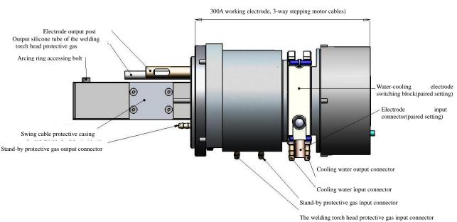
This assembly consists of an integrated converter and a front rotary output interface, completes the 300A main electrode; circulating cooling water; dual protective gas; 3-way 12-core stepper motor control cables, from relatively fixation to no wound involution states switching. Locations of all interfaces are shown above.
